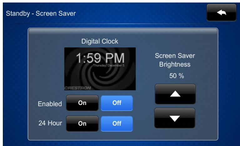
The “Standby – Screen Saver” screen provides controls to turn the *Digital Clock* screen saver **On** and **Off** as well as controls to display the time in a *24 Hour* format and to adjust the *Screen Saver Brightness*.
