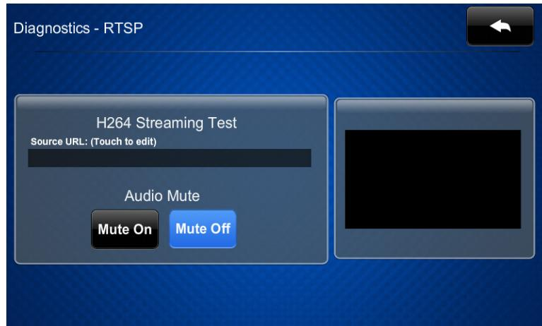
The “Diagnostics – RTSP” screen tests whether Real Time Streaming Protocol is functioning on the touch screen. Touch the area below *Source URL: (Touch to edit)* to open the on-screen keyboard. Enter the URL for an H.264 video and touch **Save**. The video is displayed on the right side of the “Diagnostics – RTSP” screen.
