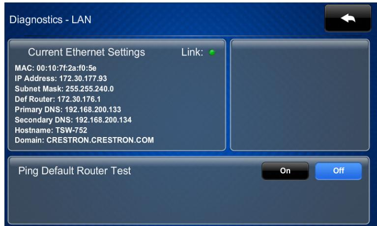
The “Diagnostics – LAN” screen displays the touch screen’s *Mac* and *IP Address*, *Subnet Mask*, *Def Router*, *Primary DNS*, *Secondary DNS*, *Hostname*, and *Domain*. This screen also contains a *Link* indicator to show the status of the Ethernet connection and controls to test the connection to the default router.
