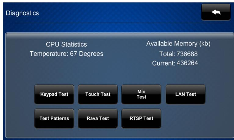
The “Diagnostics” menu displays the CPU temperature, *Available Memory* and contains controls to run a **Keypad Test**, **Touch Test**, **Mic Test**, **LAN Test**, **Rava Test**, and **RTSP Test**. In addition, there is a **Test Patterns** control to open various test pattern screens. These are explained in the paragraphs that follow.
