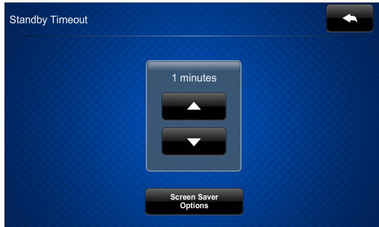
The “Standby Timeout” menu provides controls to adjust standby timeout from 0 to 120 minutes.
