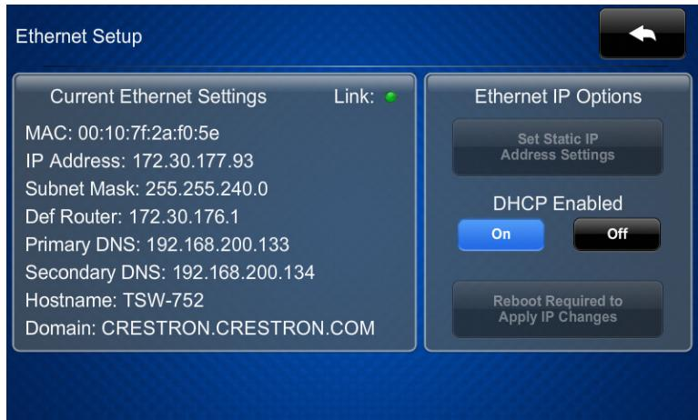
The “Ethernet Setup” menu displays the touch screen’s *Mac* and *IP Address*, *Subnet Mask*, *Def Router*, *Primary DNS*, *Secondary DNS*, *Hostname*, and *Domain*. There are controls for turning **DHCP** **On** or **Off** and, when DHCP is off, a **Set Static IP Address Settings** button, which provides access to controls which allow editing of these settings. This screen also contains a *Link* indicator to show the status of the Ethernet connection.
