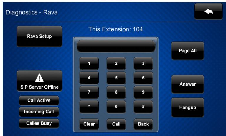
The “Diagnostics - Rava” menu provides controls for testing the use of Crestron’s Rava® SIP Intercom with the touch screen. They can be used to test projects and settings. If the intercom works but the project does not, there is an issue with the project; if the intercom does not work, there is an issue with the settings.
