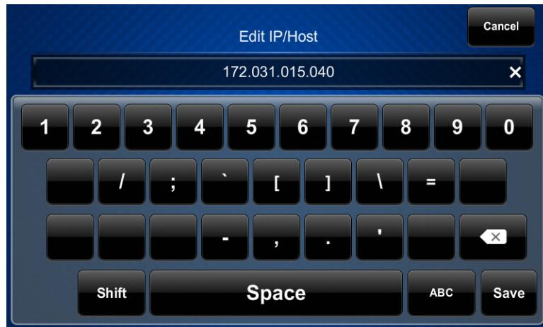
Use the keyboard to make the new entry. Touch **Cancel** to return to the “Ethernet Setup – Edit IP Table Entry” screen. Touch the “x” in the text field to clear any previous entry. Touch to delete the last digit. Touch **Save** to save a new entry and return to the “Ethernet Setup – Edit IP Table Entry” screen.
