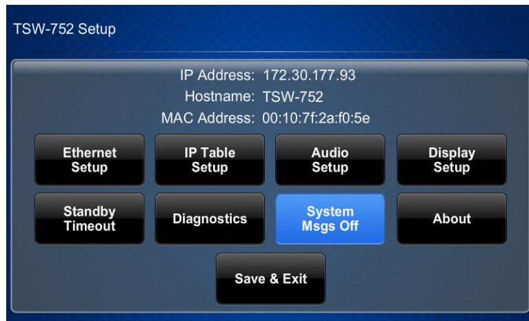
The “TSW-x52 Setup” menu is comprised of buttons for **Ethernet Setup**, **IP Table Setup**, **Audio Setup**, **Display Setup**, **Standby Timeout** and **Diagnostics**. In addition, there is a button to toggle system messages on or off, an **About** button that provides information about the touch screen and a **Save & Exit** button. The functions of each are detailed in the next section of this guide.
