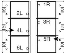
Buttons 5R and 6R are covered. When the button cap is pressed, button 5R activates.
