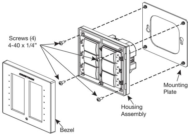
3. Attach the bezel by putting it in position over the button caps and snapping it in place.
