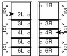
Button 4R is covered. When the button cap is pressed, button 4R activates.
