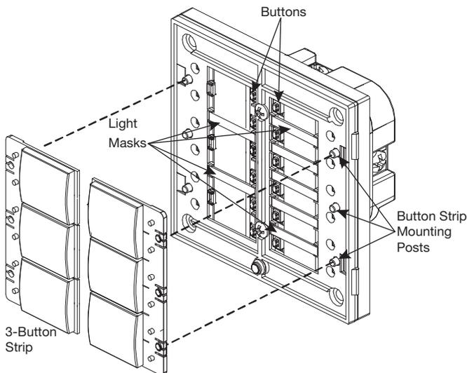
3. If the button strips need to be changed or replaced, insert the provided flat blade screwdriver into the notches and carefully pry the button strip off of the button strip mounting posts.
