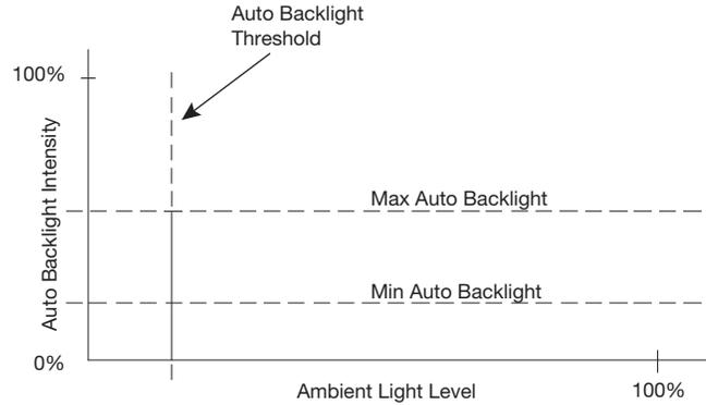
Choosing the proper values for these parameters depends on factors such as the color of the keypad, the type and placement of lighting in the room, the orientation of the room's windows with respect to the sun, and personal preference. To simplify the process, Crestron ships the Cameo keypad with preset values for the three parameters. The preset values have been selected to produce an effect that should be acceptable in many common scenarios.
