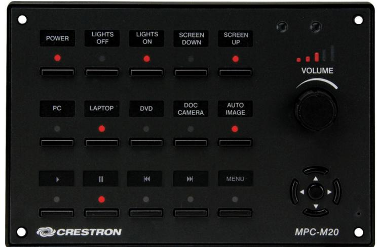
projection screen, lift, occupancy sensor, and other devices in the room. In addition to Cresnet and high-speed Ethernet, there is a bidirectional RS-232 COM port, an IR/serial port, two relays, and four input ports right on the rear panel.
