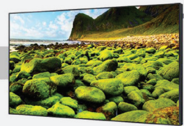
OM46D at 2,500 nit Using 220 W
