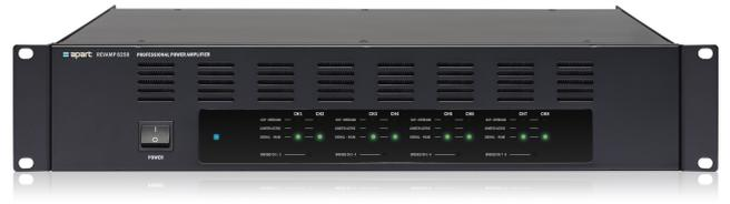
This 8-channel bridgeable power amplifier is probably the most versatile class-D amplifier in the range. Combined with a pre-amplifier or matrix the REVAMP8250 can be used to create 8 zones in mono, 4 zones in stereo, even 4 bridged mono or 2 bridged stereo systems can be created. The amplifier has an intelligent variable speed cooling fan built-in to keep the unit cool at all times.
