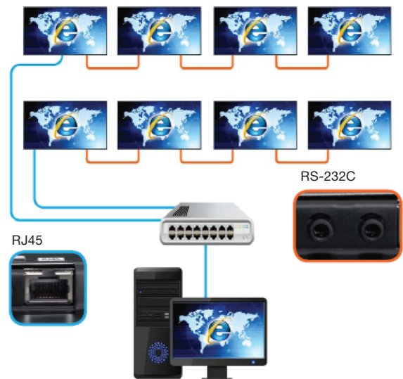
Figure 4. Samsung ME65B and ME75B LED displays enable RJ45 and RS-232 connectivity simultaneously.
