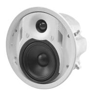
The speaker assembly is shipped with a detachable paper cover fitted over the transducers inside the bezel. This protective cover protects the drivers from damage during installation and also serves as a paint cover, allowing convenient spray painting to match interior décor. A powder-coated perforated steel grille is supplied, and easily installed once the desired Tap Selector and Full-Range/ High-Pass switches have been set.
