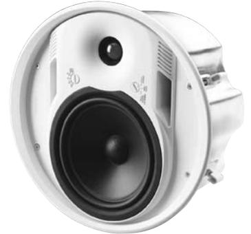
The speaker assembly is shipped with a detachable plastic cover fitted over the transducers inside the bezel. This protective cover protects the drivers from damage during installation and also serves as a paint cover, allowing convenient spray painting to match interior décor. A powder-coated perforated steel grille is supplied, and easily installed once the desired Tap Selector and Full-Range/High-Pass switches have been set.
