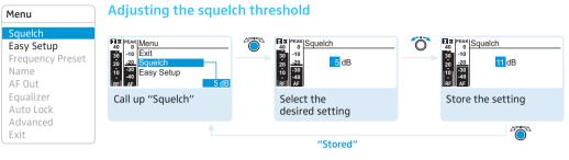
Adjustment range: 5 to 25 dB $\mu V$ , adjustable in 2-dB steps, can be switched off
