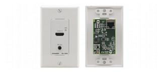
The SV-306 is a wall plate for HDMI and IR signals. The unit is part of the SummitView<sup>™</sup> media room solution and converts the signals to a twisted pair signal to connect to the SV-552 BrainBox<sup>™</sup> processor/controller.
