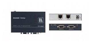
The TP-202 is a twisted pair transceiver for computer graphics video signals with resolutions VGA up to UXGA or HDTV signals. It takes a twisted pair signal and converts it back into a computer graphics video signal or HDTV signal available on two 15-pin HD outputs and simultaneously re-transmits the original twisted pair signal to another compatible receiver.
