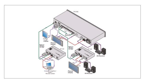
signals.System Range (Twisted Pair) - Up to 100 meters (300 feet).Cable (Twisted Pair) - UTP (unshielded twisted pair) or STP (shielded twisted pair) such as CAT 5.Power Connect™ SystemOnly the TP-310A needs to be connected to a power source when the devices are within 150 feet (50 meters) of each other.Worldwide Power Supply - 100-240V AC.Standard 19" Rack Mount Size - 1U. Rack "ears" included.Matched Transmitters: TP-45, TP-121, TP-205A, TP-210A
