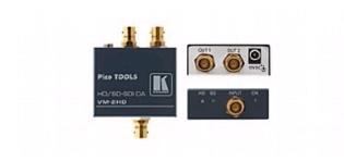
The VM-2HD is a high performance distribution amplifier for SDI (SMPTE 259M and SMPTE 344M) and HD-SDI (SMPTE 292M) signals. It will take one input, provide reclocking and equalization and distribute the signal to two identical outputs.
