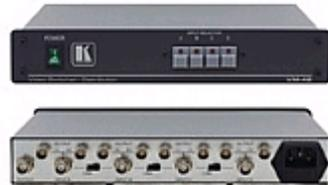
The Kramer VM-42 is high performance distribution amplifier and switcher for composite video signals. It can be used as a 4x1 vertical interval switcher with each input becoming a 1:2 DA or it can take one input, provide correct buffering and isolation, and distribute the signal to eight identical outputs.
