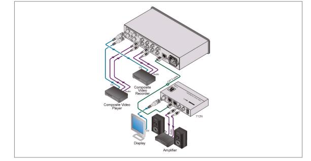
Termination - 75 Ohm. Recessed Level (Gain) & EQ (Peaking) Controls Audio Level Control.System Range (Twisted Pair) - More than 500 meters (1500 feet). Greater distances possibledepending on signal resolution and cable. Cable (Twisted Pair) -UTP (unshielded twisted pair) such as CAT 5.Worldwide Power Supply - 100-240V AC. Desktop Size - Two units can be rack mounted side-by-side in a 1U rack space.
