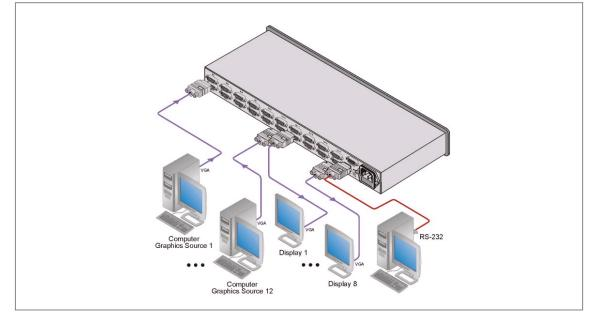
switches as presets to be recalled and executed when needed. Take Button - Execute multiple switches all at once. Front panel lock. Control - RS-232 with looping (K-Router™ Window® - based software is included), Ethernet & IR Remote (included). Worldwide Power Supply - 100-240 V AC. Standard 19" Rack Mount Size - 1U. Rack "ears" included.
