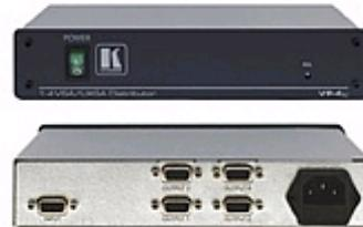
The VP-3xl, **VP-4xl**, & VP-5xl are high performance distribution amplifiers for computer graphics video signals with resolutions ranging from VGA through UXGA and higher. It takes one input, provides correct buffering and isolation, and distributes the signal to three, four, or five identical outputs.
