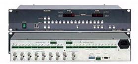
The VS-1002xI, VS-1202xI, and VS-1602xI are high performance matrix switchers for composite video and balanced stereo audio signals. Switching during the vertical interval ensures glitch-free switching with genlocked sources.
