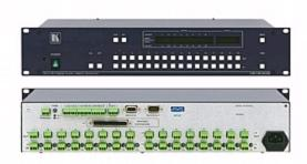
The VS-1616AD is a high performance matrix switcher for digital audio (S/PDIF & AES/EBU) signals. It can route any or all inputs to any or all outputs simultaneously on 110 ohm twisted pair cable.
