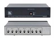
The VS-21 switches three identical channels simultaneously. It can serve as a high performance switcher for component video (YUV or RGB) signals. It switches any one of two component signals to a single component output. The VS-21 can also switch composite video with two audio channels, independent composite video channels or any other combination.
