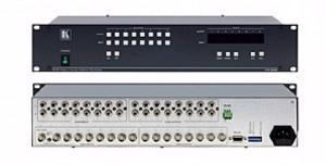
The VS-626, VS-824, and VS-828 are high performance matrix switchers for composite video and unbalanced stereo audio signals. Switching during the vertical interval ensures glitch-free switching with genlocked sources.
