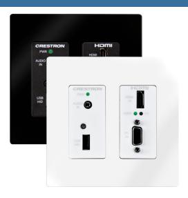
assessed and managed through the DM-TX-200-2G, ensuring reliable operation by instructing sources to output only the resolutions and formats that can be handled by the displays and system wiring.
