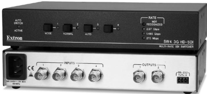
The Extron SW4 3G HD-SDI is a four input, dual output switcher for multi-rate SDI digital video. This broadcast-quality switcher accepts SDI and HD-SDI signals at all common serial digital video data rates up to 3G-SDI including SMPTE 259M, SMPTE 292M, and SMPTE 424M, as well as embedded audio, ancillary ID and metadata information. The SW4 3G HD-SDI is ideal for applications that require the switching of a wide range of high resolution digital video signals.
