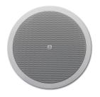
The Apart CM8E is a 2-way 100 volt built-in ceiling loudspeaker. The loudspeaker has an 8" woofer, a 1" coaxial tweeter and a high quality 100 volt loudspeaker line transformer with multiple power taps.
