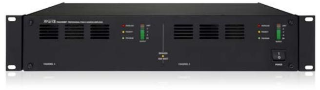
The PA2240BP is a bridgeable and ultra-reliable 2-channel 100 volt power amplifier that can be used in all your big 100 volt projects. It can be configured as a 2-channel amplifier (2 x 240 watts) or it can be bridged into a 1 x 480 watts power amplifier if you need to power a big group of loudspeakers up to 480 watts.
