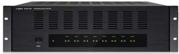
REVAMP1680 is a professional 16-channel digital power amplifier with 16 x 100 watts output power @ 4 ohms, but the unit is also bridgeable to 8 x 200 watts @ 8 ohms. This 3 rack units high amplifier with very high channel separation also has a dual analog power supply with toroidal power transformers. The standby power consumption is very low, less than 0.5 watts!
