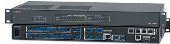
DMP 128 Plus C AT 12x8 ProDSP™ Digital Matrix Processor with AEC and Dante • Eight channels of AEC - acoustic echo cancellation • Dante audio networking for a wide range of expansion capabilities
