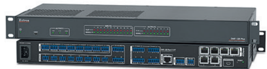
DMP 128 Plus C V AT 12x8 ProDSP™ Digital Matrix Processor with AEC, VoIP, and Dante • Eight channels of AEC - acoustic echo cancellation • Up to eight VoIP lines that can support generic SIP 2.0 - RFC 3261 • VoIP configuration via onboard web page separates AV and IT workflows • Dante audio networking for a wide range of expansion capabilities
